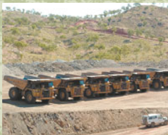
Figure 8 - Open pit mining trucks parked at the ‘GO’ line
